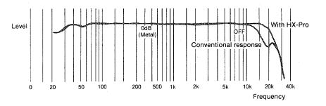
When recording, a bias current according to the tape type used is applied to the recording head as well as the music signal to improve the distortion rate. Furthermore, the extreme high frequency content of a music signal can actually act as bias, adding to the deck's own bias signal to produce over-bias conditions. The result is the deterioration of the high frequency components of the music signal.
