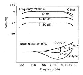
With cassette tapes, the most noticeable form of noise is high frequency hiss. To reduce this hiss noise, the unit is equipped with the newer Dolby C noise reduction system in addition to the older Dolby B NR. Either type of noise reduction may be selected with the DOLBY NR selector.
